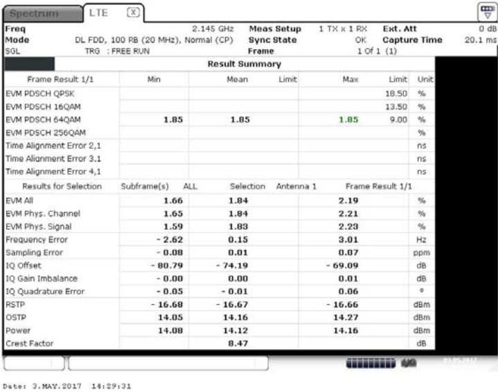
Figure 10 I/Q constellation table with I/Q error – 64QAM (2145.0 MHz) (20MHz Channel BW)
