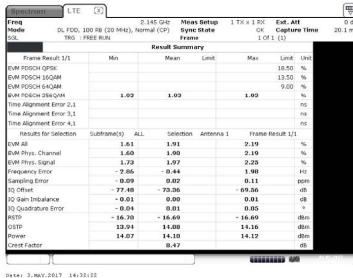
Figure 12 I/Q constellation table with I/Q error – 256QAM (2145.0 MHz) (20MHz Channel BW)
