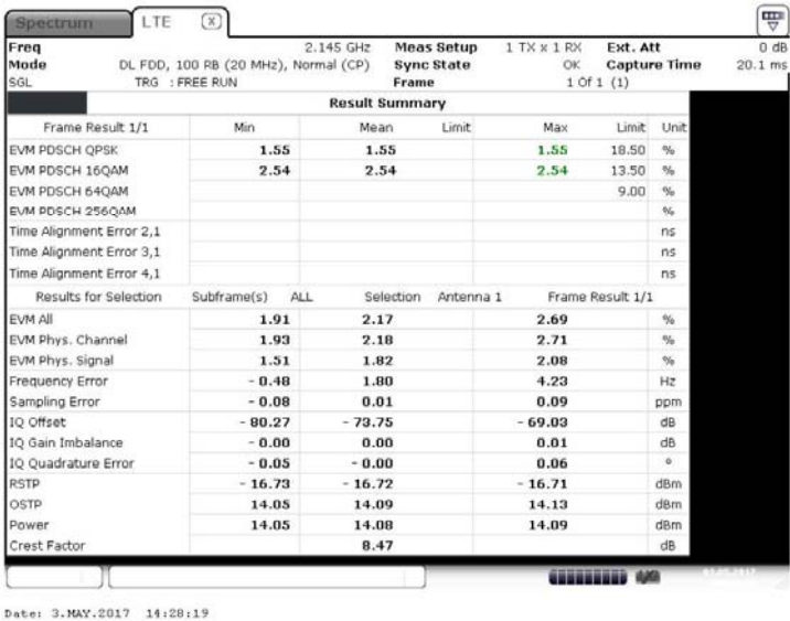
Figure 8 I/Q constellation table with I/Q error – 16QAM (2145.0 MHz) (20MHz Channel BW)
