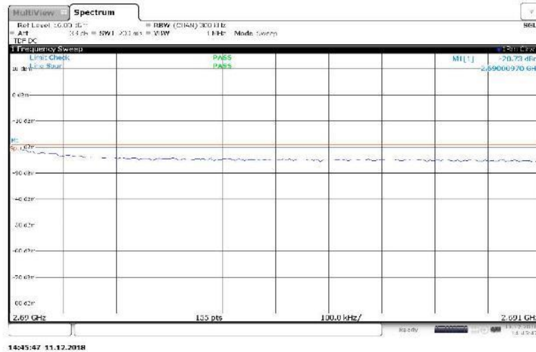
Figure 154 Spurious Emissions (Upper Band Edge) – 16QAM (2667.5 MHz, 2682.5 MHz, 2x15 MHz Channel BW)
