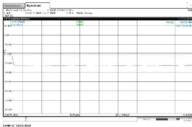
Figure 174 Spurious Emissions (2.676 GHz – 3 GHz) – QPSK (2645 MHz, 2665 MHz, 2x20 MHz Channel BW)
