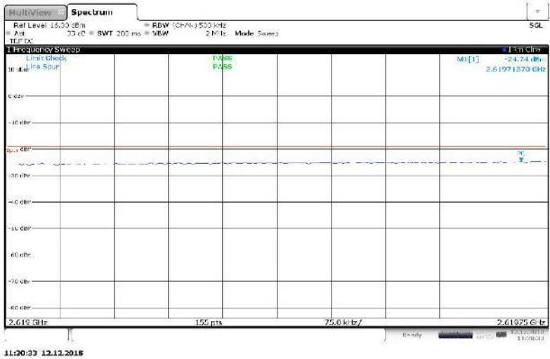
Figure 189 Spurious Emissions (Lower Band Edge) – 256QAM (2630 MHz, 2650 MHz, 2x20 MHz Channel BW)
