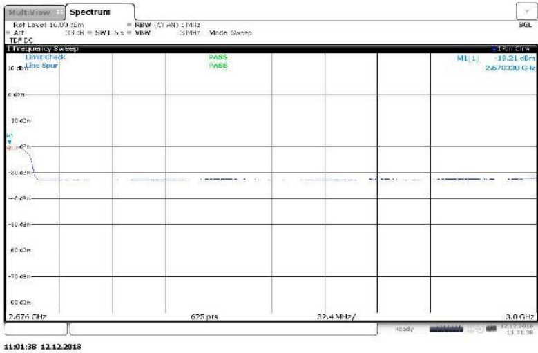
Figure 186 Spurious Emissions (2.676 GHz – 3 GHz) – 64QAM (2645 MHz, 2665 MHz, 2x20 MHz Channel BW)
