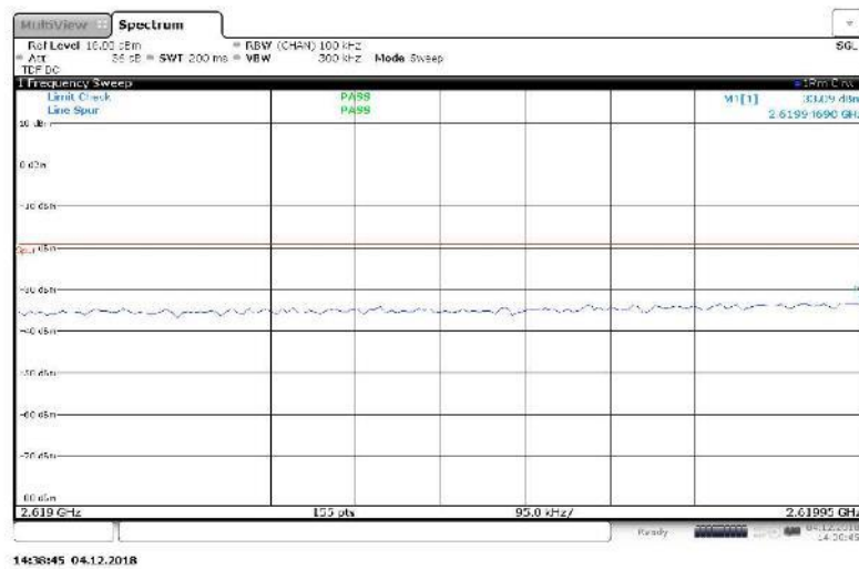
Figure 33 Spurious Emissions (Lower Band Edge) – 16QAM (2625 MHz, 10 MHz Channel BW)
