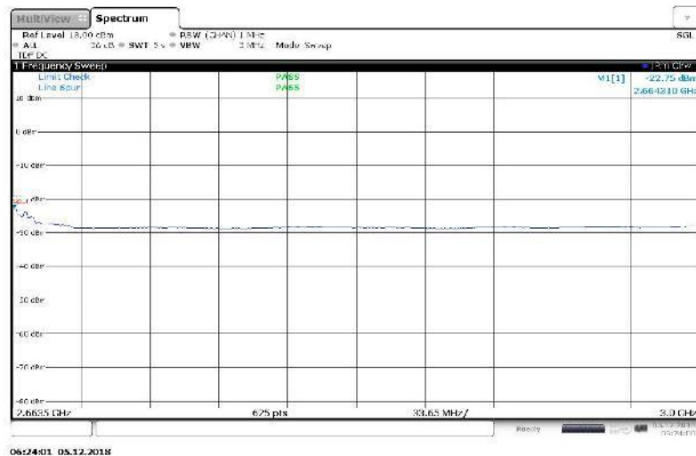
Figure 66 Spurious Emissions (2.6635 GHz – 3 GHz) – 64QAM (2655 MHz, 15 MHz Channel BW)
