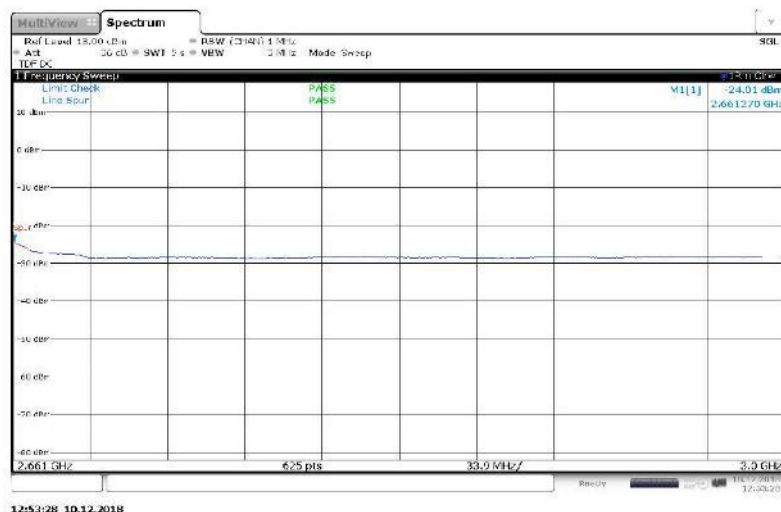
Figure 102 Spurious Emissions (2.661 GHz – 3 GHz) – QPSK (2652.5 MHz, 2657.5 MHz, 2x5 Channel BW)
