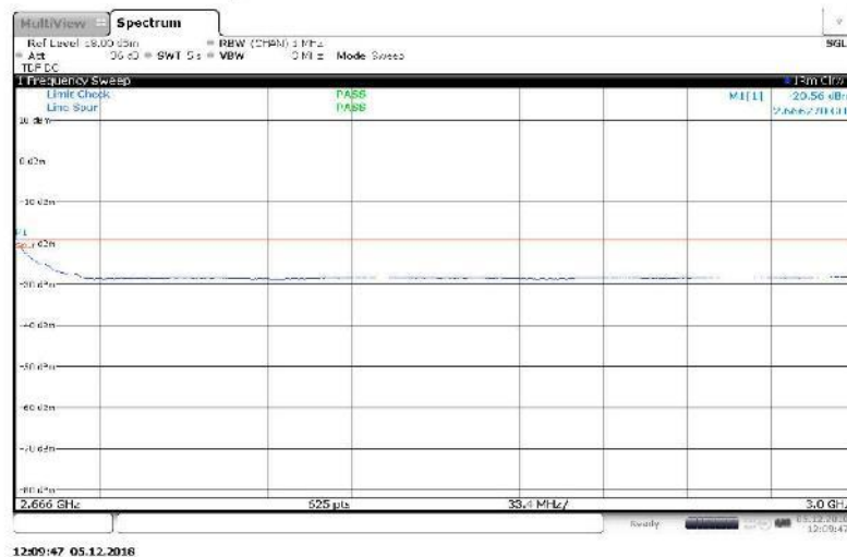
Figure 78 Spurious Emissions (2.666 GHz – 3 GHz) – QPSK (2655 MHz, 20 MHz Channel BW)
