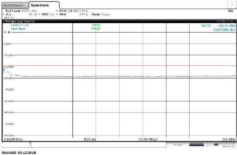
Figure 54 Spurious Emissions (2.6635 GHz – 3 GHz) – QPSK (2655 MHz, 15 MHz Channel BW)
