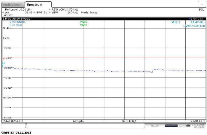
Figure 4 Spurious Emissions (Upper Band Edge) – QPSK (2687.5 MHz, 5 MHz Channel BW)
