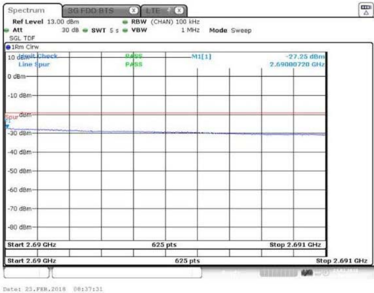
Figure 88 Spurious Emissions (Upper Band Edge) – 256QAM (2685 MHz, 10 MHz Channel BW)
