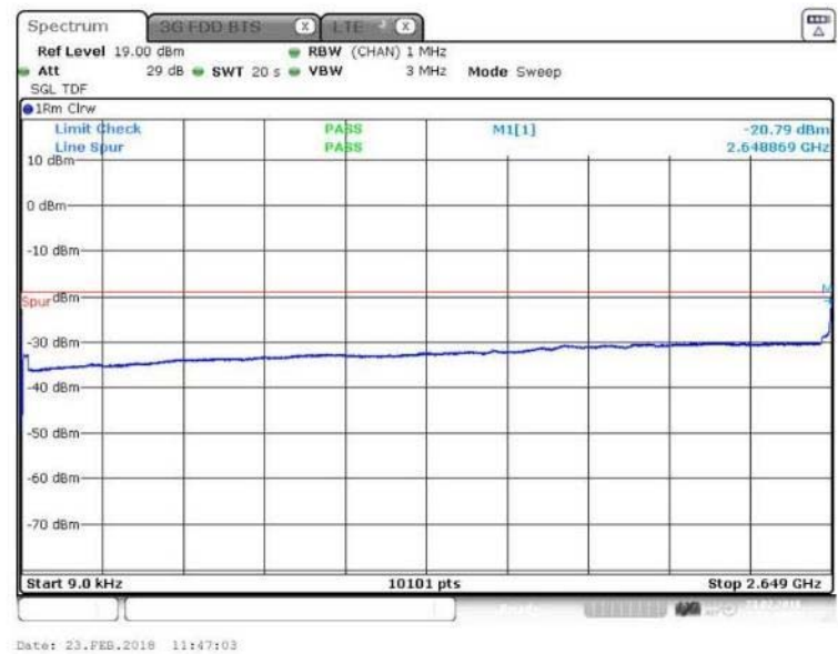
Figure 71 Spurious Emissions (9kHz – 2.649 GHz) – QPSK (2655 MHz, 10 MHz Channel BW)
