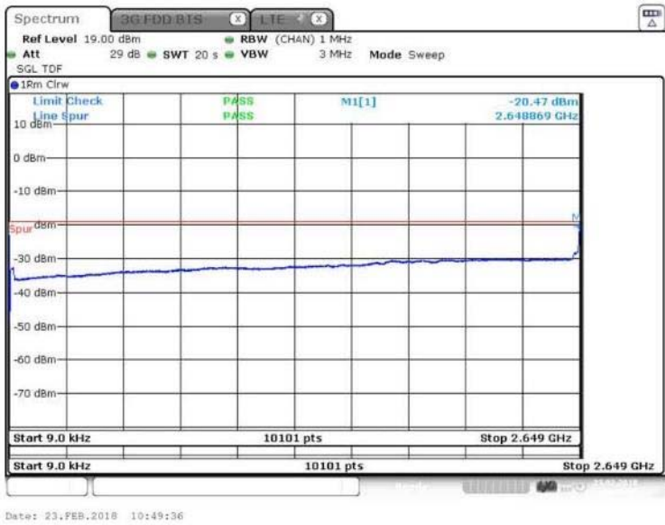
Figure 83 Spurious Emissions (9kHz – 2.649 GHz) – 64QAM (2655 MHz, 10 MHz Channel BW)
