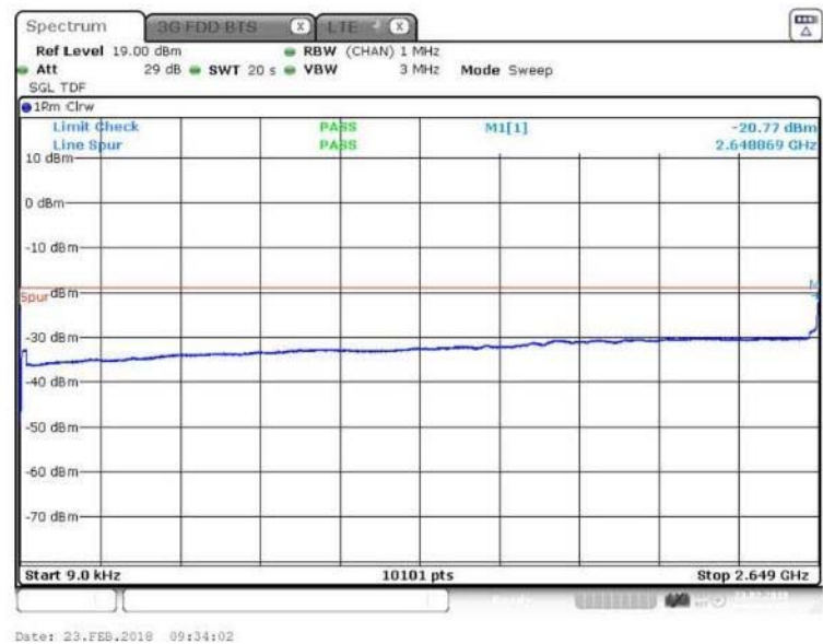
Figure 89 Spurious Emissions (9kHz – 2.649 GHz) – 256QAM (2655 MHz, 10 MHz Channel BW)
