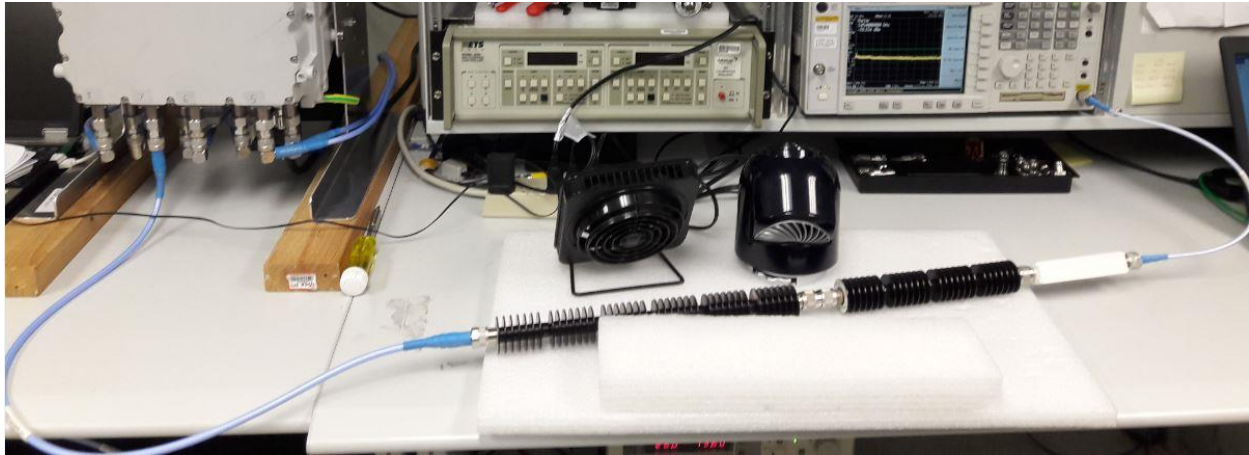
Setup for 9kHz to 150kHz and 150kHz to 20MHz Measurements
