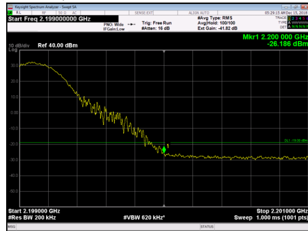
LTE20 Top Channel UBE 2199MHz to 2201MHz
