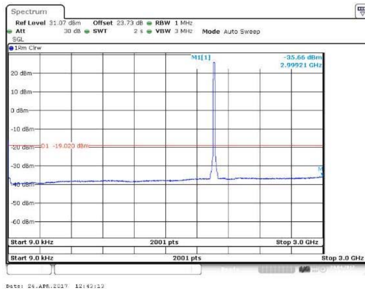
Figure 79 Spurious Emissions (9kHz – 3GHz) - QPSK (1962.5 MHz) (20MHz Channel BW)
