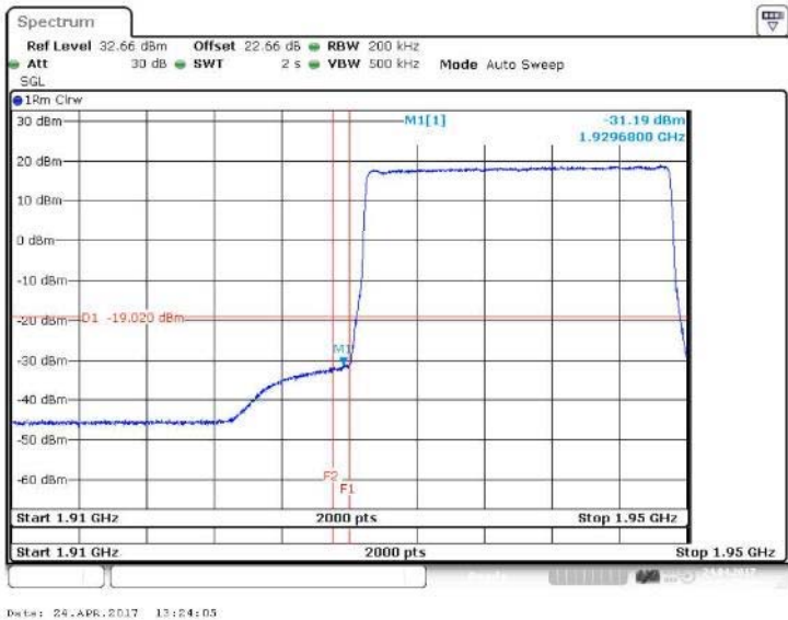
Figure 73 Spurious Emissions (Lower Band Edge) – 256QAM (1940.0 MHz) (20MHz Channel BW)
