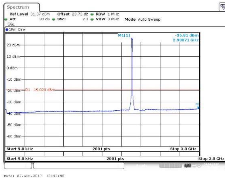
Figure 83 Spurious Emissions (9kHz – 3GHz) – 16QAM (1962.5 MHz) (20MHz Channel BW)
