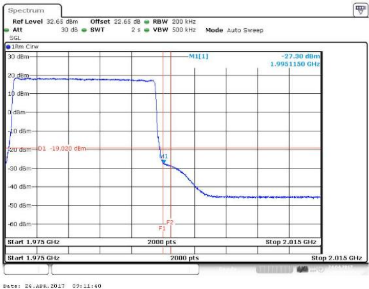
Figure 90 Spurious Emissions (Upper Band Edge) – 256QAM (1985.0 MHz) (20MHz Channel BW)
