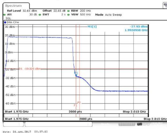
Figure 78 Spurious Emissions (Upper Band Edge) – QPSK (1985.0 MHz) (20MHz Channel BW)
