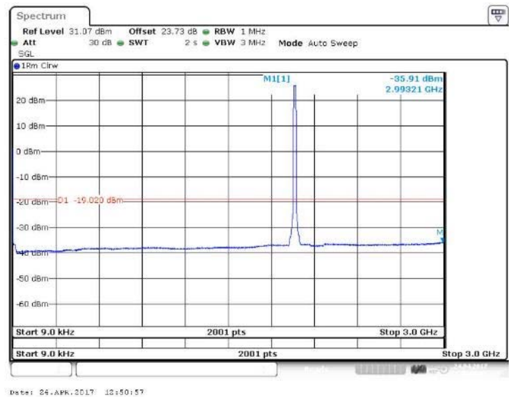
Figure 87 Spurious Emissions (9kHz – 3GHz) – 64QAM (1962.5 MHz) (20MHz Channel BW)
