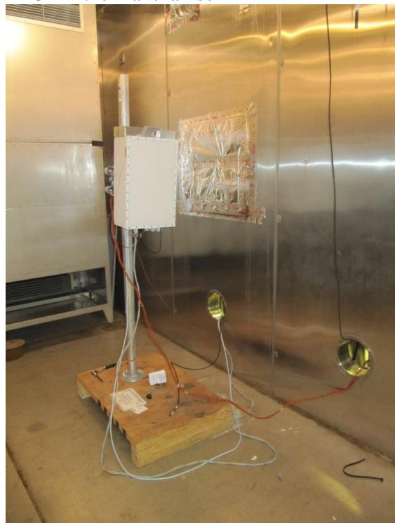
**Horn Antenna (outside of thermal chamber)**
