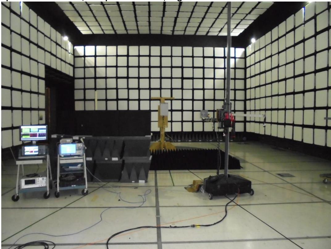
**Radiated Spurious Setup for 40-100 GHz**
