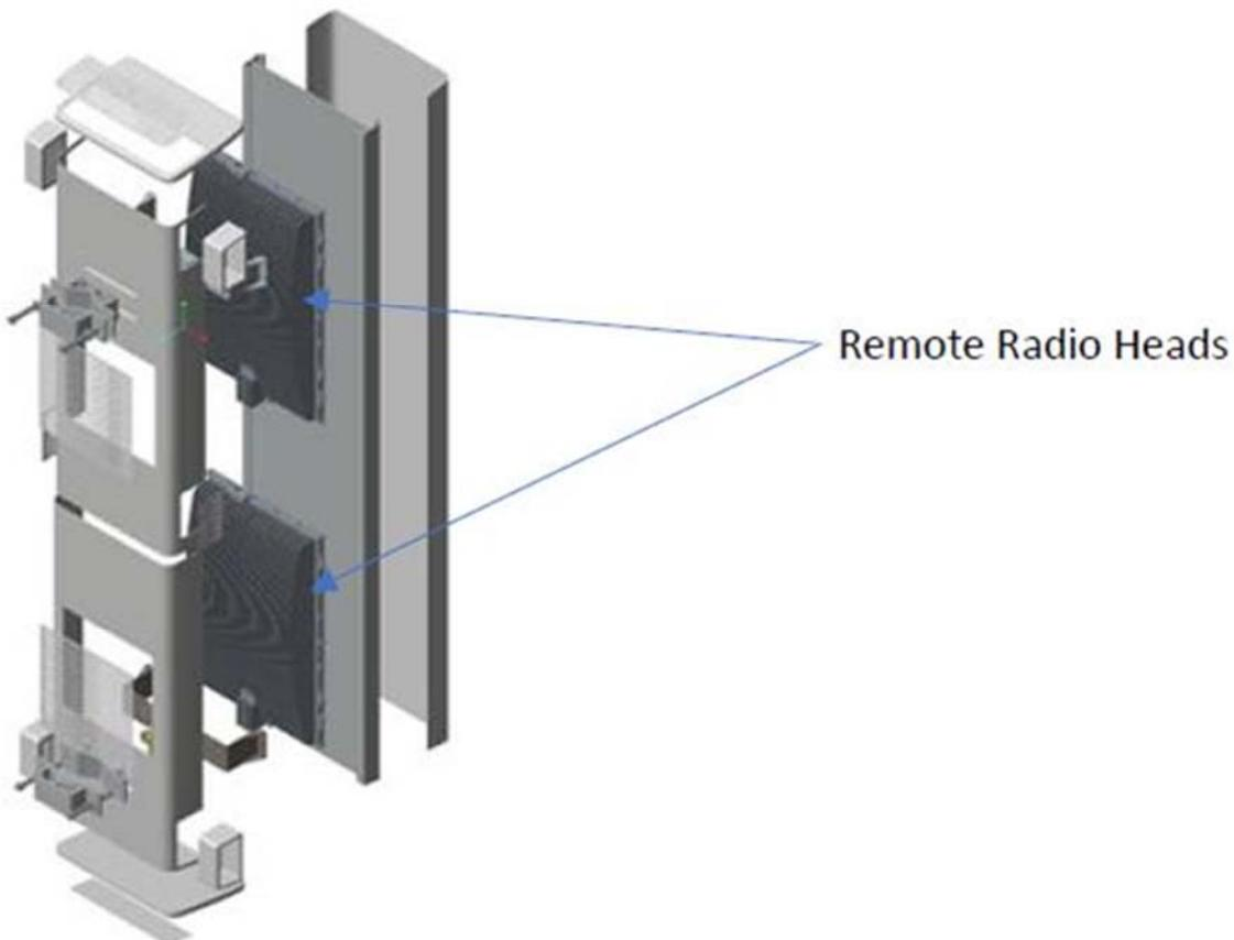
Each radio contains 16 transmitters. Each transmitter in the AAIB and AAFB is rated at 6.25W, and in the AAIC each transmitter is rated at 9.375W. Each radio will consist of a chassis, spine card, baseband/RF boards, filter, and antenna, stacked as shown below.
