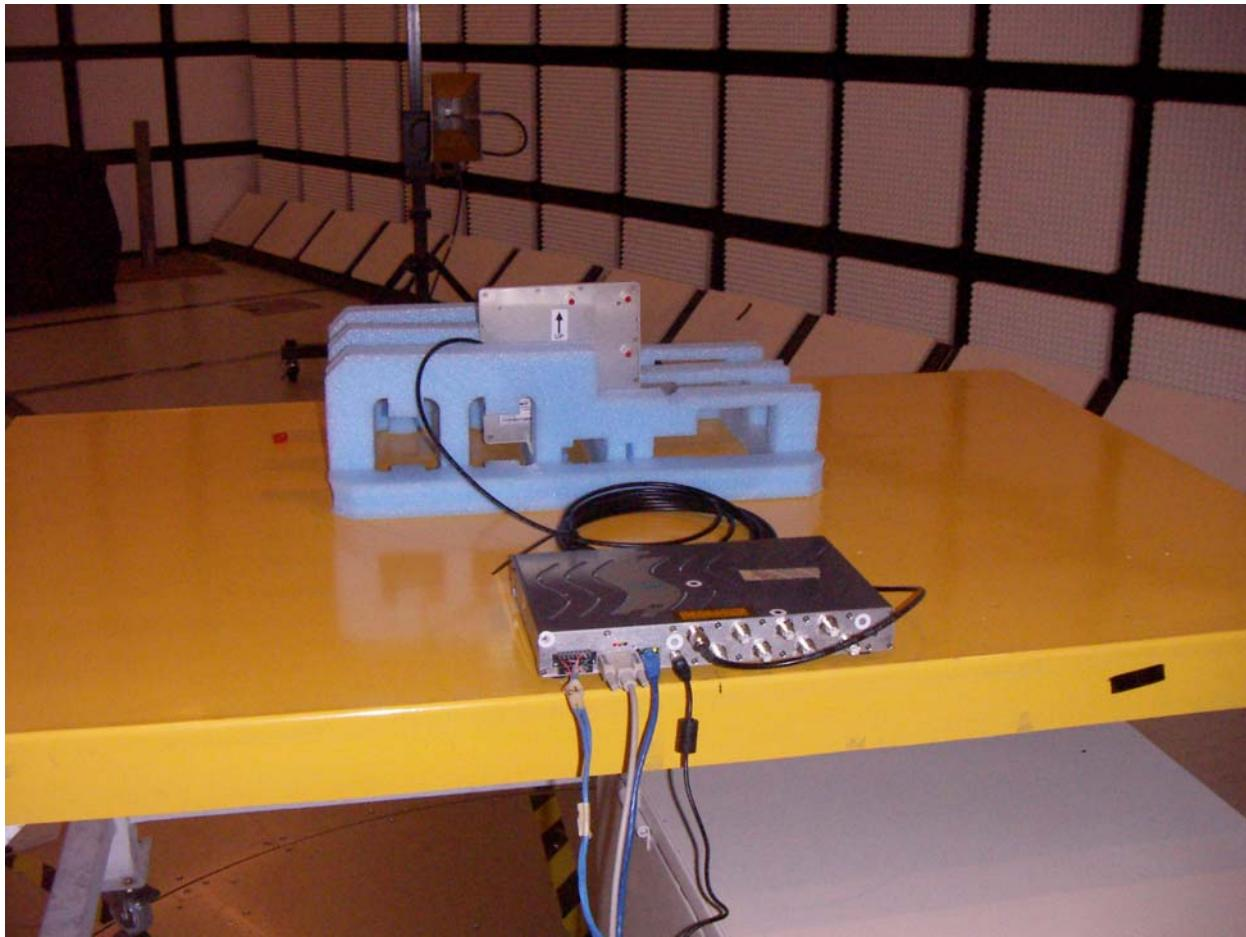
**RADIATED RF MEASUREMENT SETUP NEW CASE**
