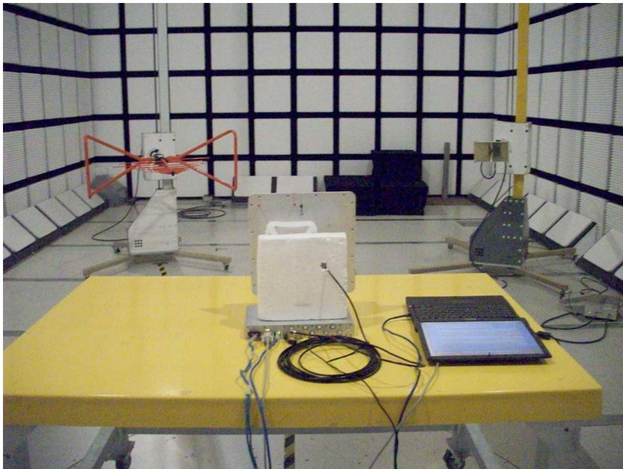
**POWERLINE CONDUCTED EMISSIONS MEASUREMENT SETUP**
