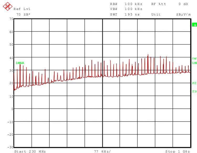
At following frequencies the highest radiation levels were found during the preliminary radiated emission test:
