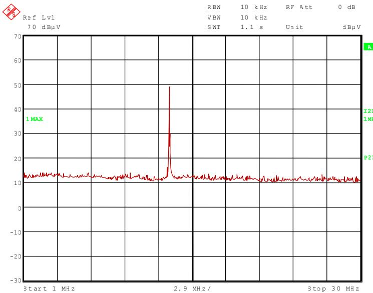
The following frequency was found inside the 13.533 to 13.567 MHz band according to FCC 47 CFR Part 15 section 15.225 [3]:
