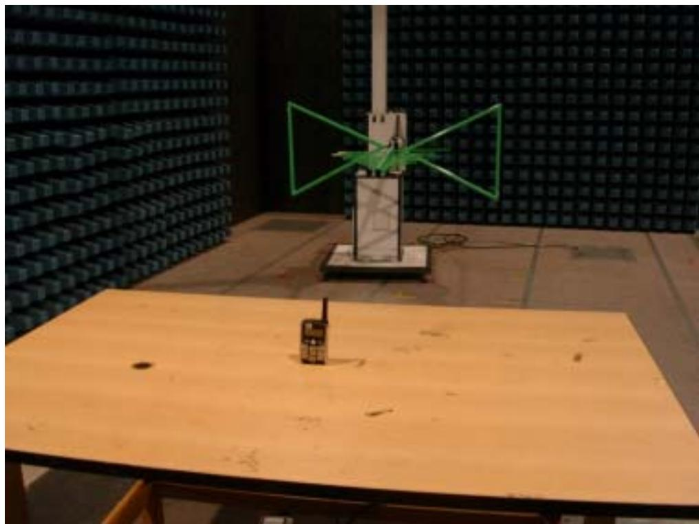
Radiated Spurious Emission Test Setup Above 1GHz
