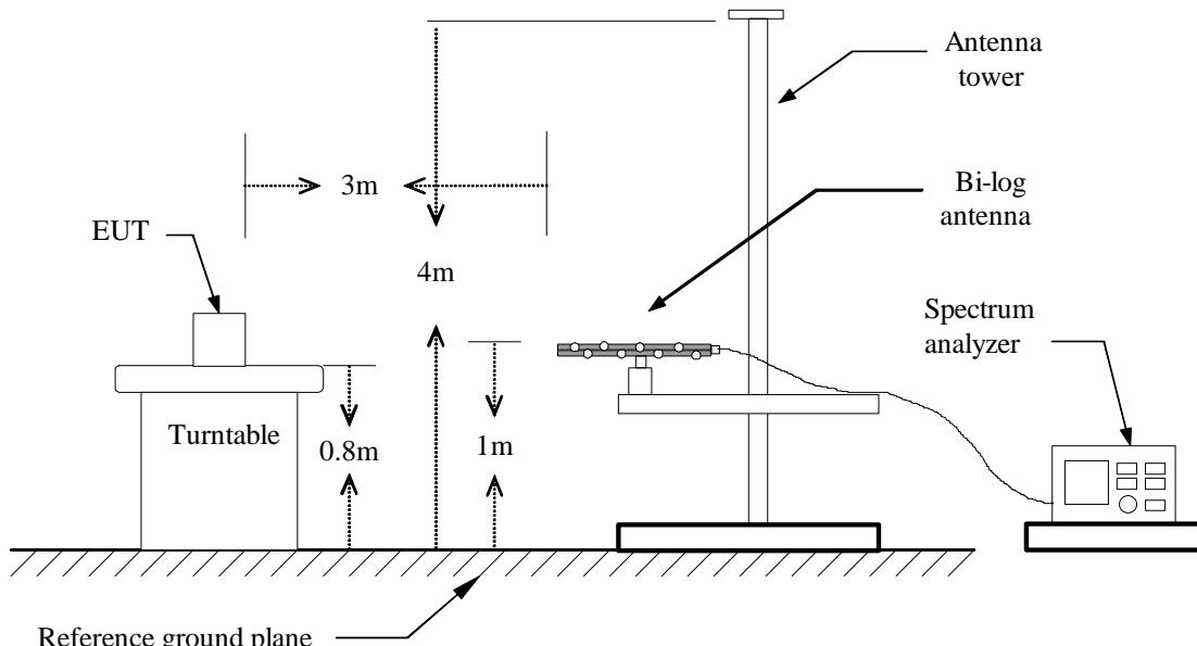
**Above 1 GHz**
