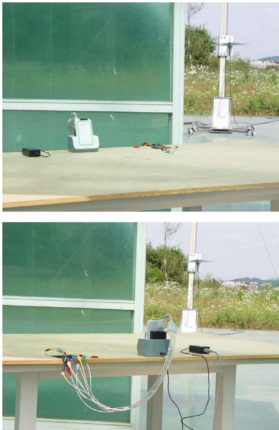
Figure 14 : Photo of Radiated emission test setup(Recording mode)
