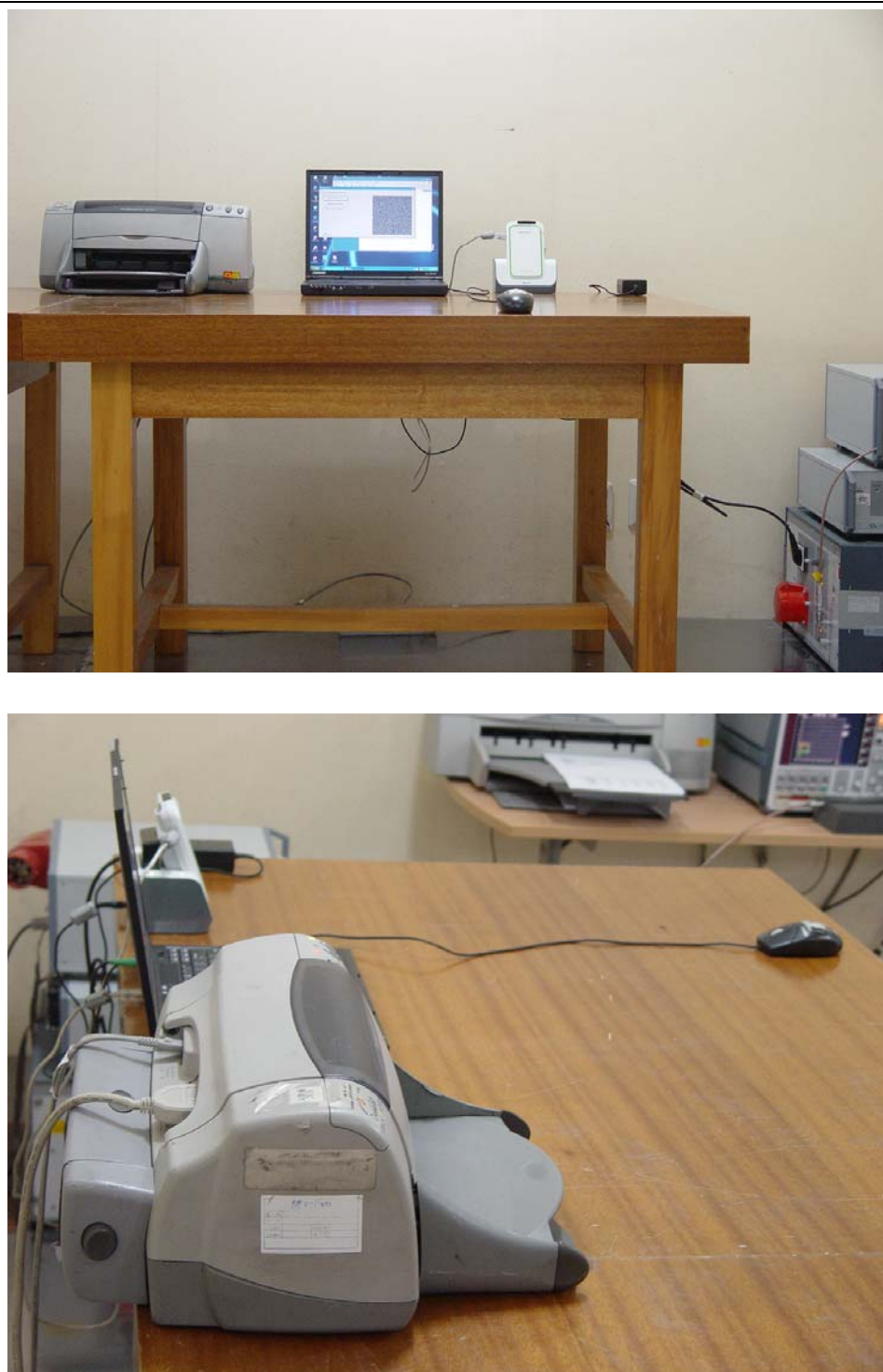
Figure 1 : Conducted Emission Test Setup
