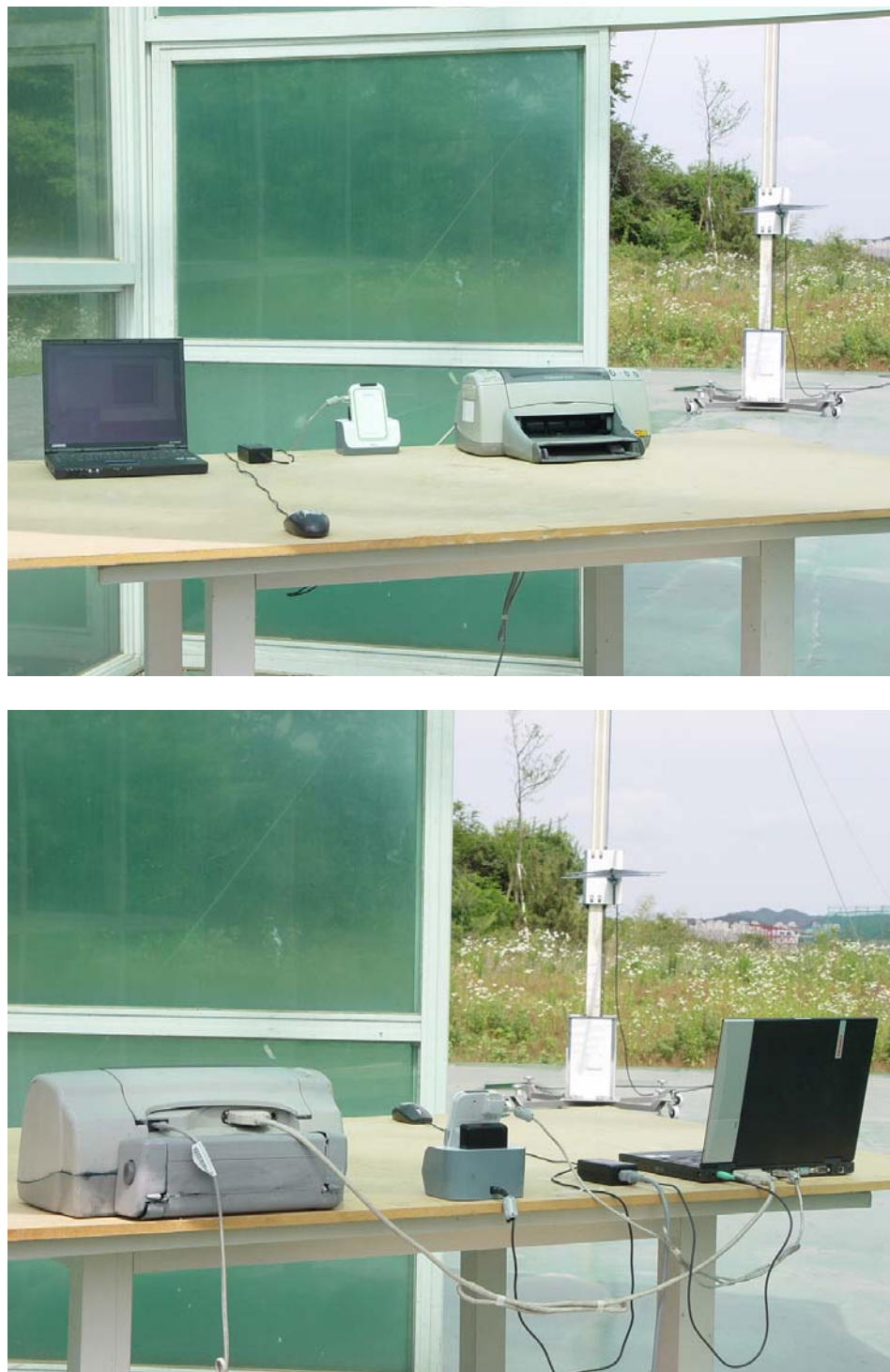
Figure 13 : Photo of Radiated emission test setup(Download mode)
