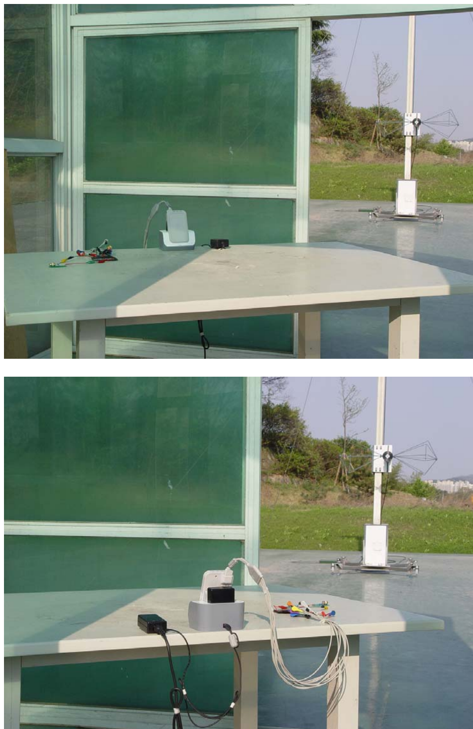
Figure 14 : Photo of Radiated emission test setup(Recording mode)
