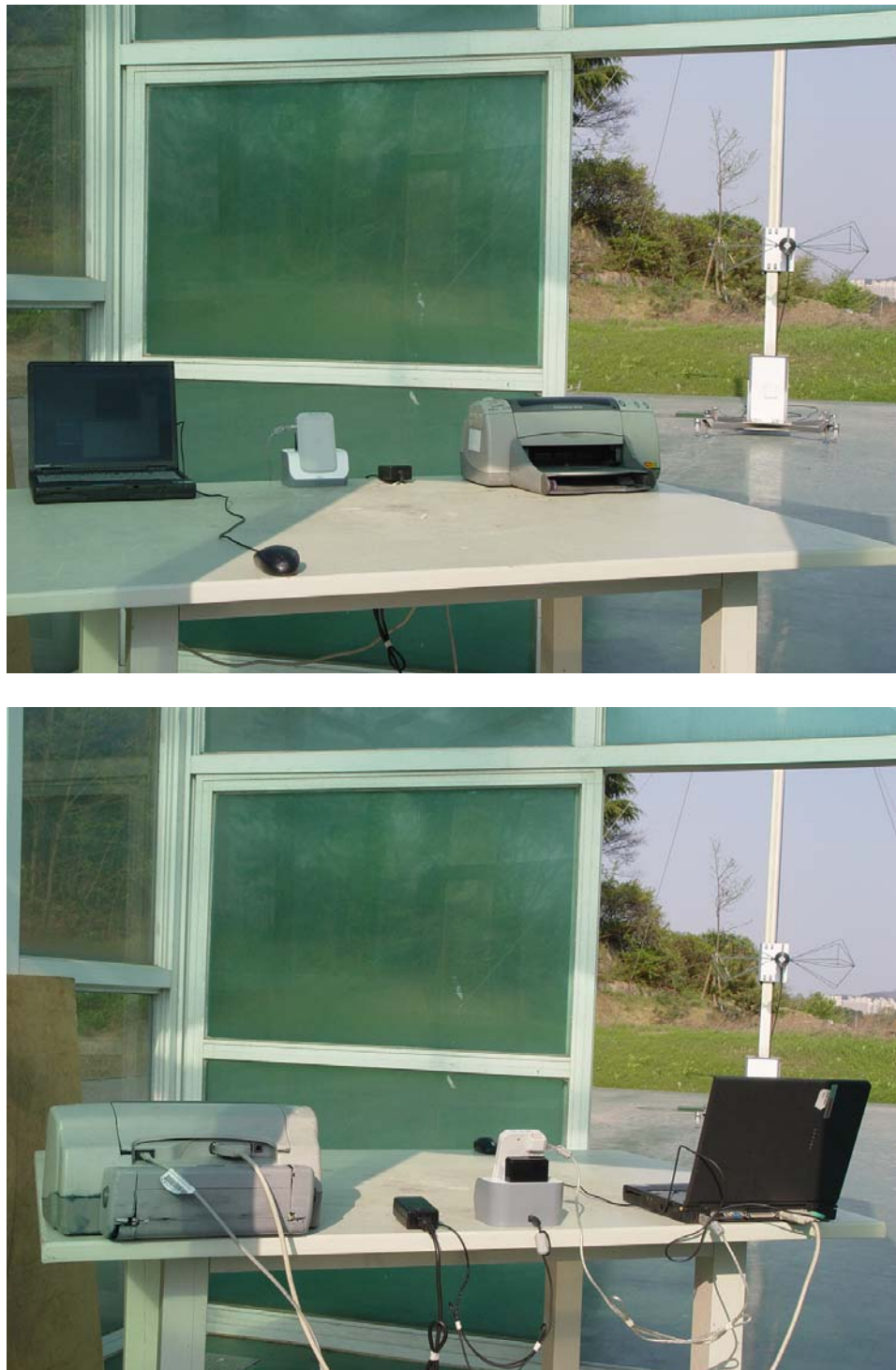
Figure 13 : Photo of Radiated emission test setup(Download mode)
