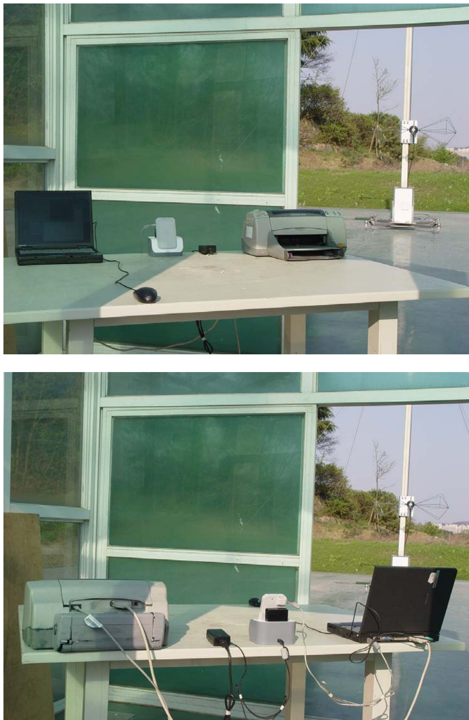
Figure 13 : Photo of Radiated emission test setup(Download mode)
