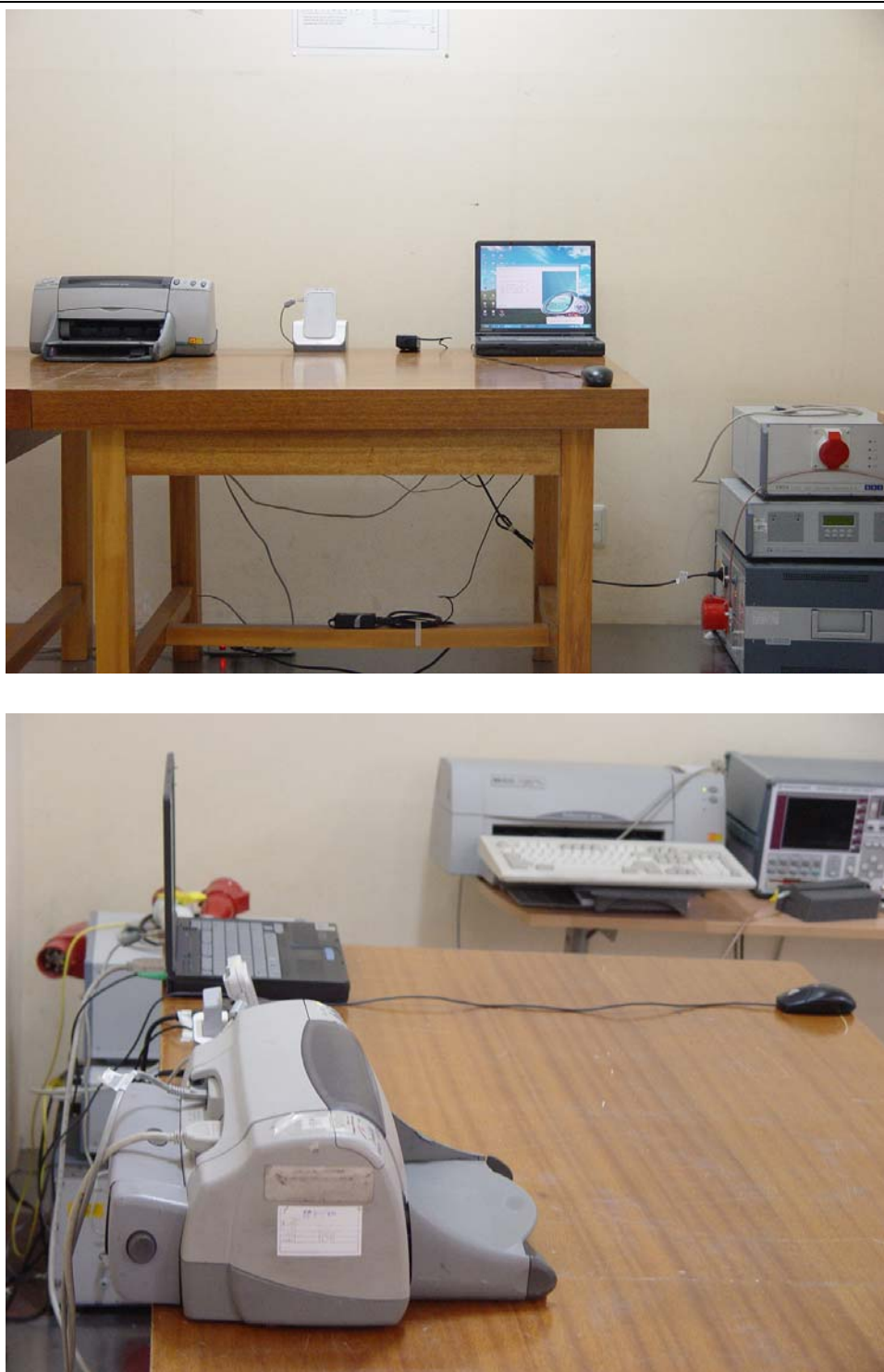
Figure 1 : Conducted Emission Test Setup
