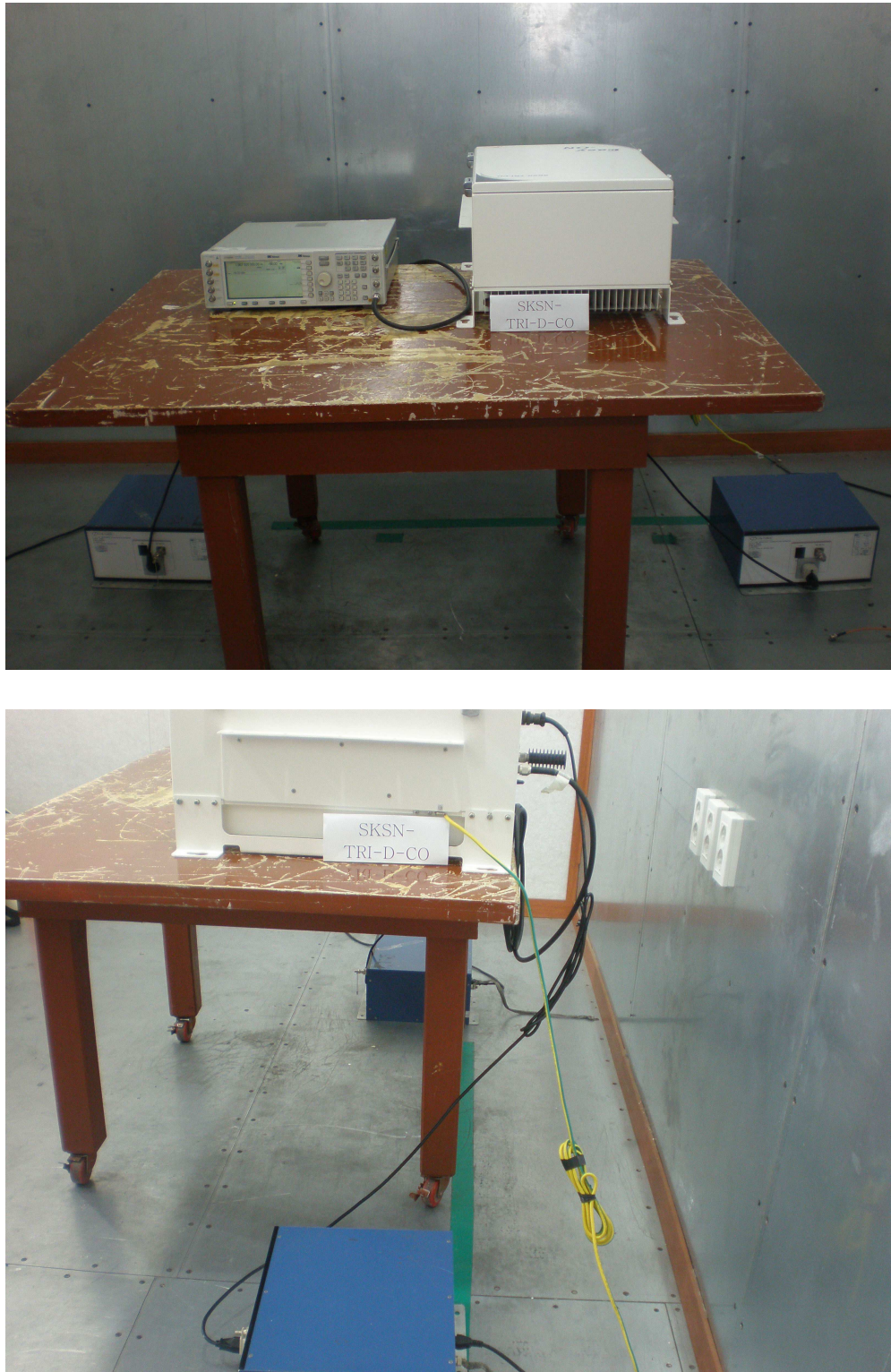
Figure 1 Test Setup for Conducted Emissions
