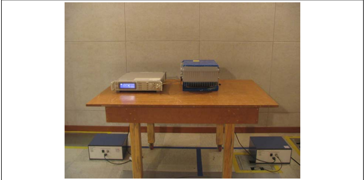
Figure 1 Test Setup for Conducted Emissions
