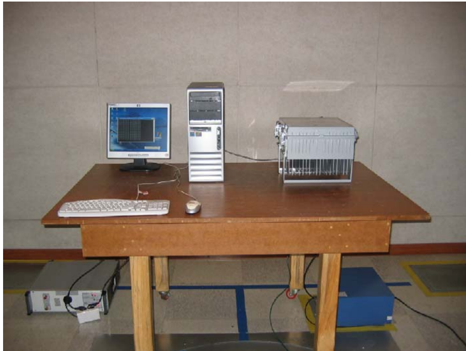
Figure 1 Test Setup for Conducted Emissions
