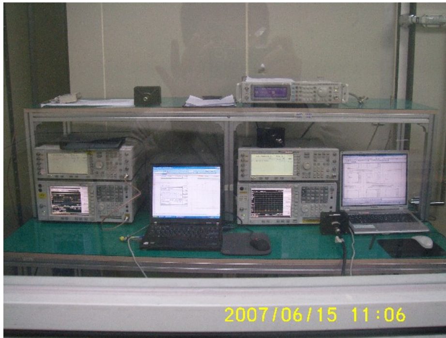
Figure 4 Test setup for Conducted Measurement
