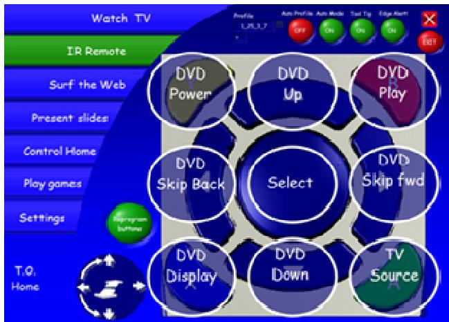
**3. IR Blasting:** When you press a key that has an IR code associated with it, such as "DVD Power", the POD will send a very powerful IR blast into the room. Reflections from the walls in your room should be sufficient to control any IR device in your room. There is also a jack in the back of the POD that will support standard IR blaster cables.
