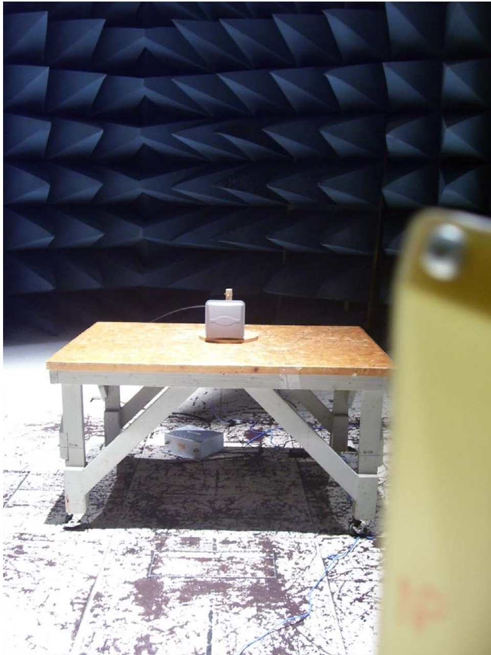
Photograph 5. Test Equipment and setup for various Radiated Measurements – 19dBi
