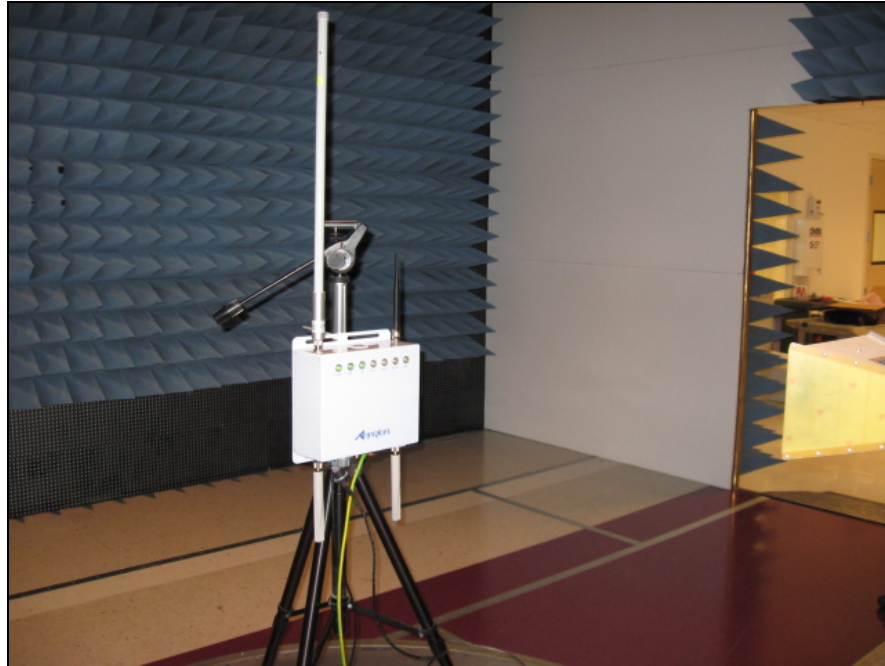
Photograph 6. Test Equipment and setup for various Radiated Measurements, 1m Distance Setup
