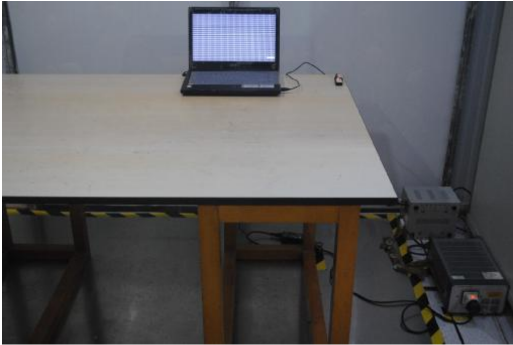
Radiated emission test view
