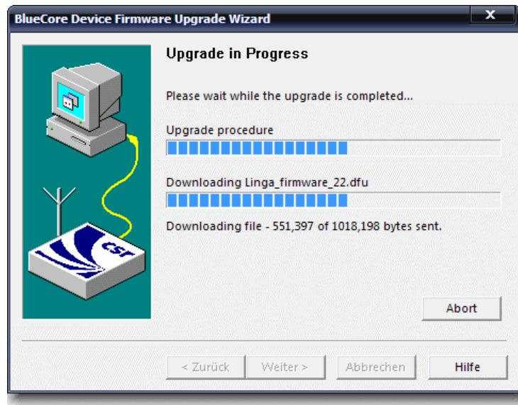
The updating process will take about two minutes. Do not shut down your PC, the B-Speech Linga or interrupt the connection while the upgrade is in progress. This can cause serious damage to the device.
