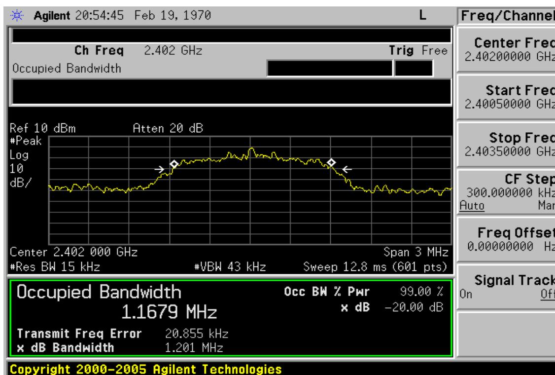
**20dB Bandwidth Test Data CH-Mid**
