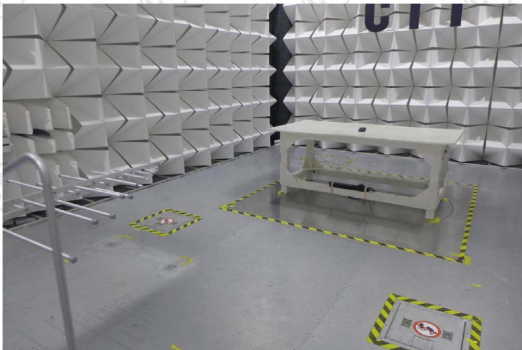
Radiated emission Test Setup-1(Below 1GHz)
