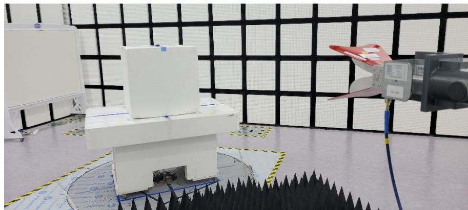
**3) RADIATED RF MEASUREMENT SET-UP (Axis)**
