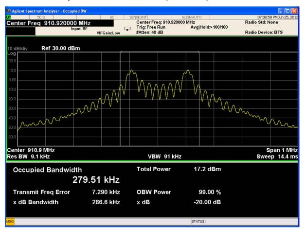
20 dB bandwidth: 286.6 kHz99 % bandwidth: 279.51 kHz
