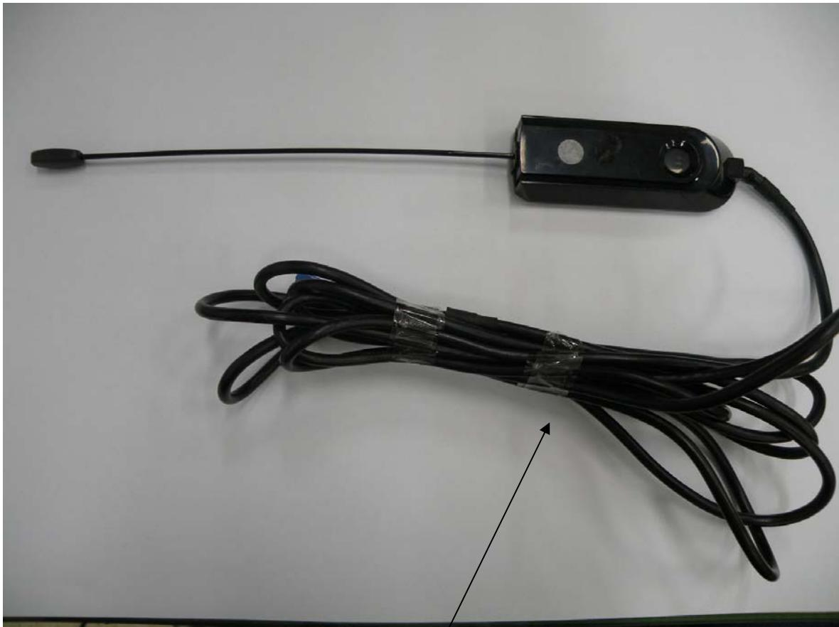
Power Line Connected to Car battery
