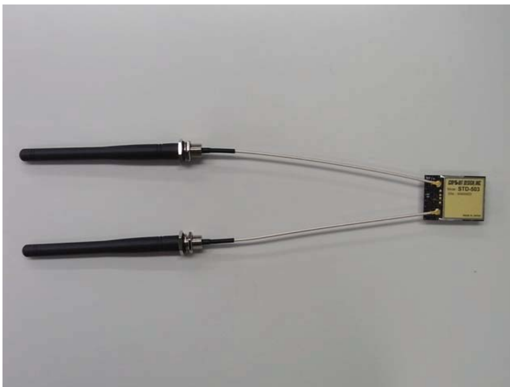
W/Sleeve antenna (water proof)
