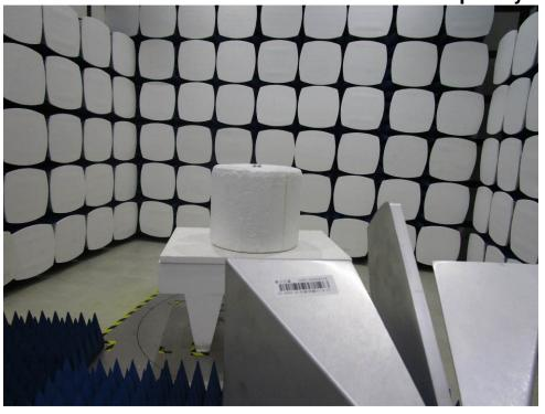
1.3 Radiated Emissions Test Setup
