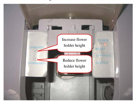
8) Put the flower into flower holder, close the cover and make the petal flat. Press "UPWARDS' to increase the height flower holder, the distance between the top point of the petal and the bottom of the cartridge head is about  $2.0\pm0.5$ mm. Printing when finish adjusting.
