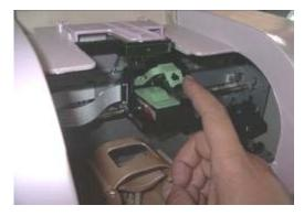
4.4. Press "RESET", the cartridge plate will back to original place.
