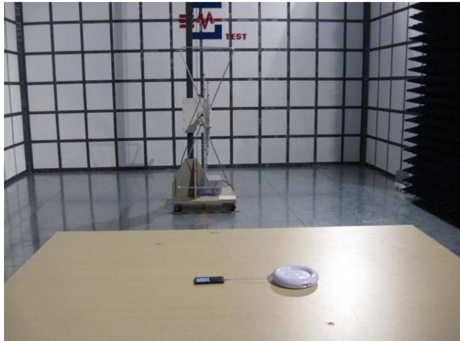
Radiation Emission Test Setup (Above 1GHz)
