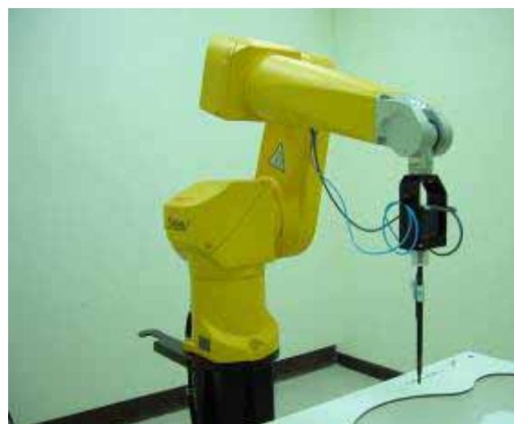
Fig. 5.2 Probe Setup on Robot
