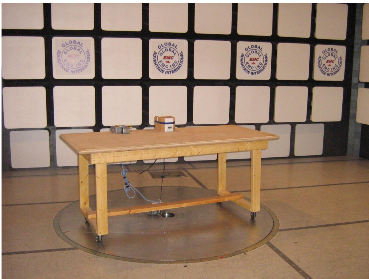
Figure 1 – EUT Radiated emission setup
