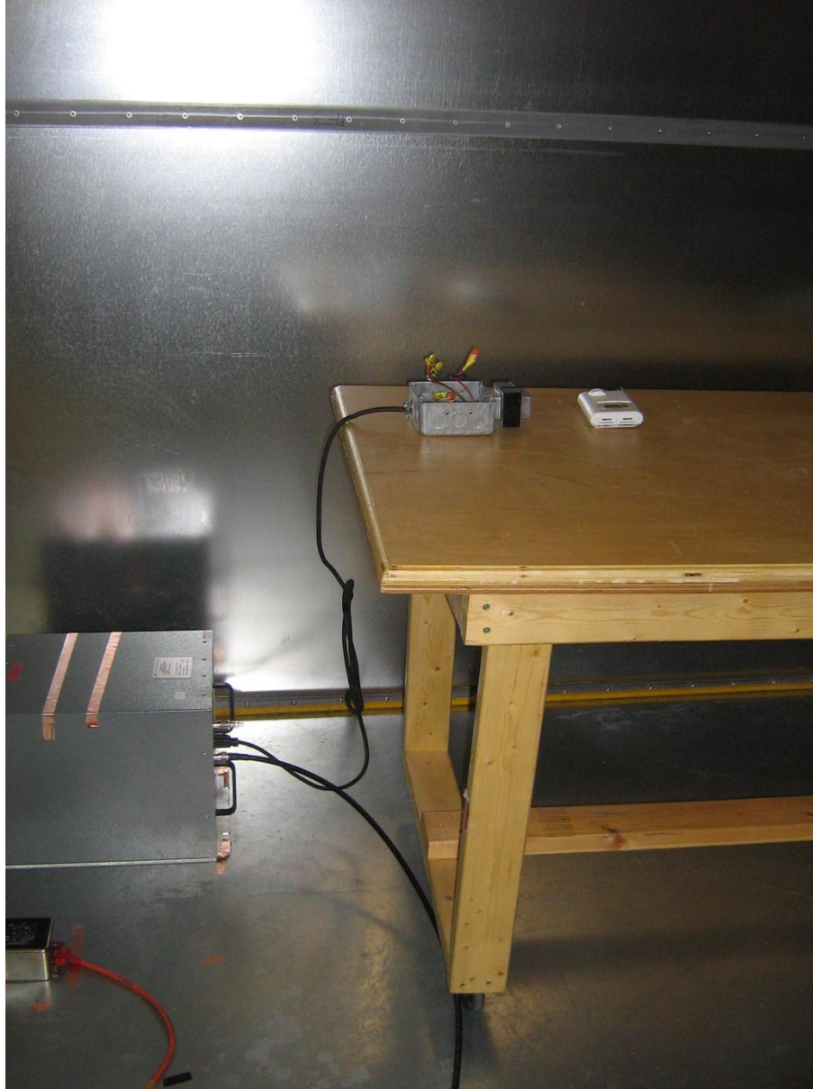
Figure 2 – Conducted emission setup
