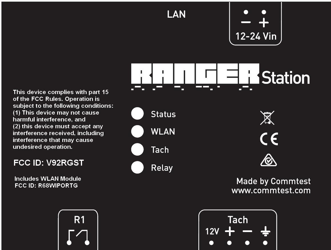
Label is printed on 8B35 0.25mm Polycarbonate backed by Scotch 467 Adhesive.
