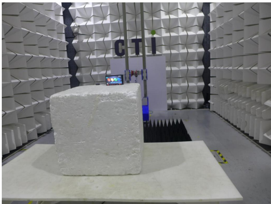
Radiated spurious emission Test Setup-3(Above 1GHz)
