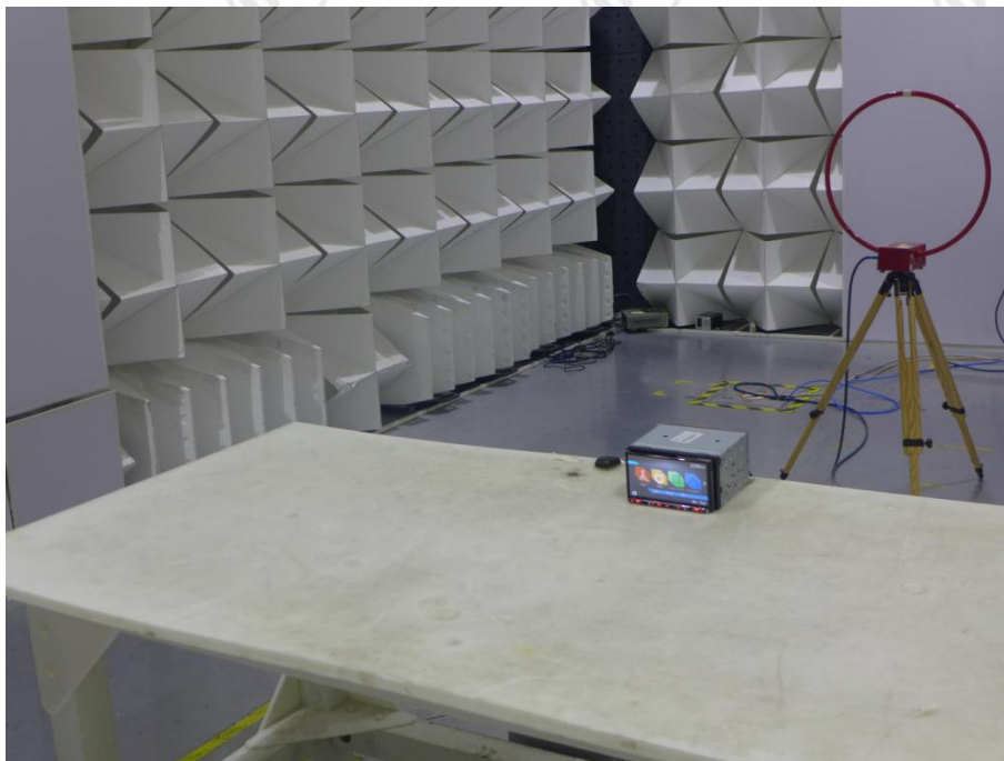
Radiated spurious emission Test Setup-1(Below 30MHz)
