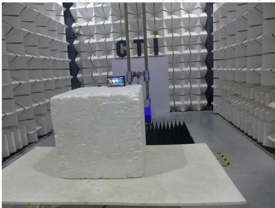
Radiated spurious emission Test Setup-3(Above 1GHz)
