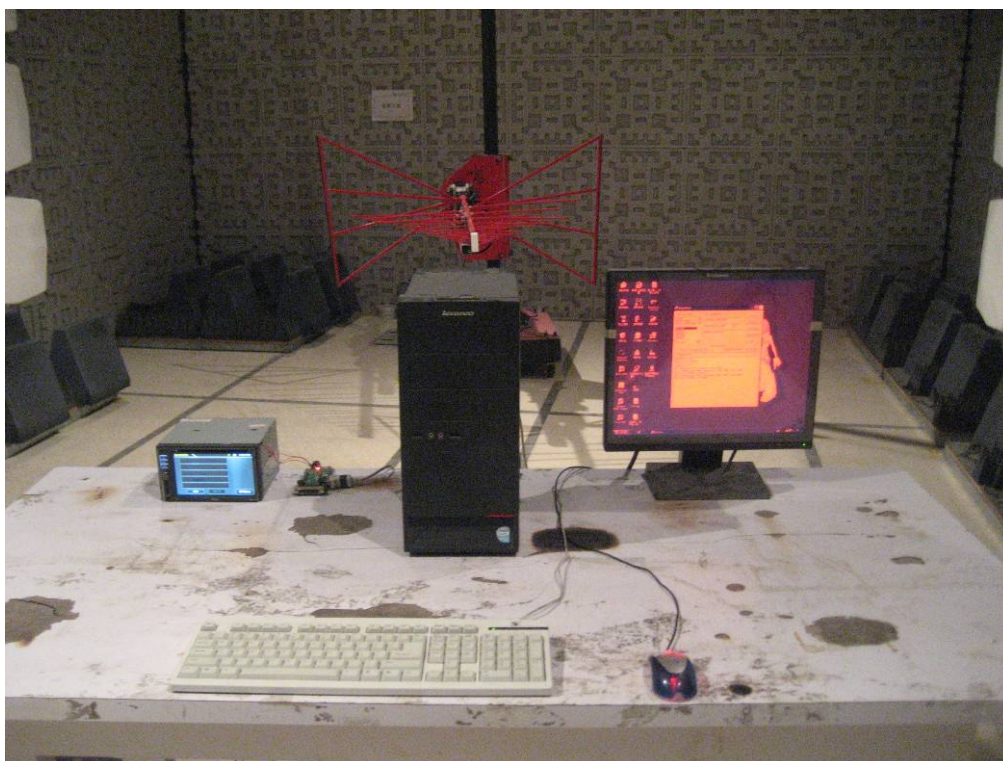
TEST SETUP OF RADIATED EMISSION (30MHz-1GHz)
