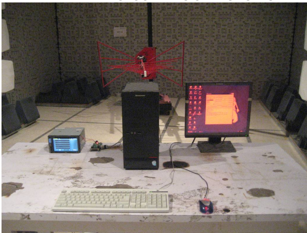
TEST SETUP OF RADIATED EMISSION (30MHz-1GHz)
