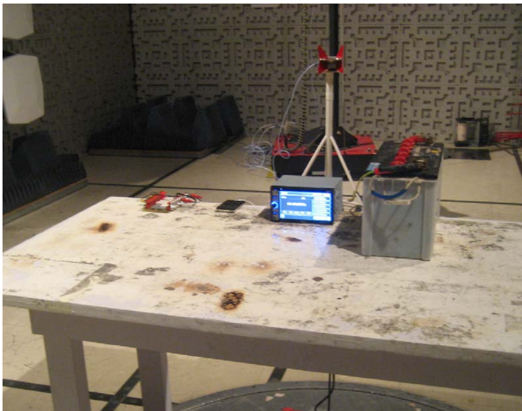
TEST SETUP OF RADIATED EMISSION (above 1GHz)
