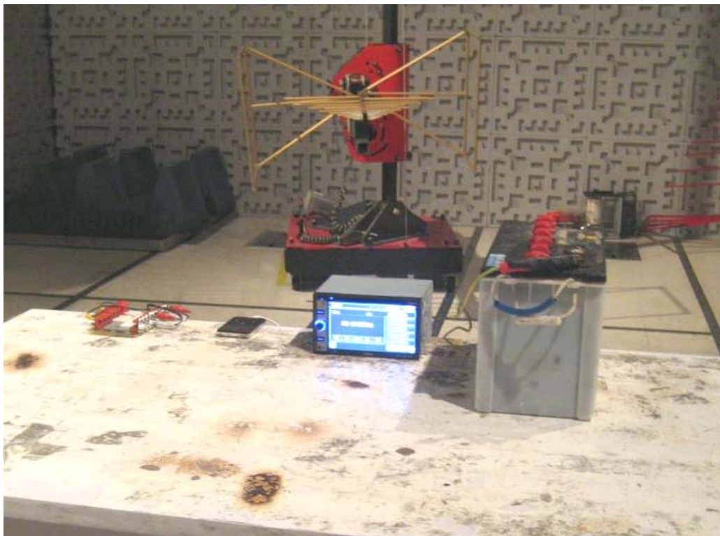
TEST SETUP OF RADIATED EMISSION (30MHz-1GHz)
