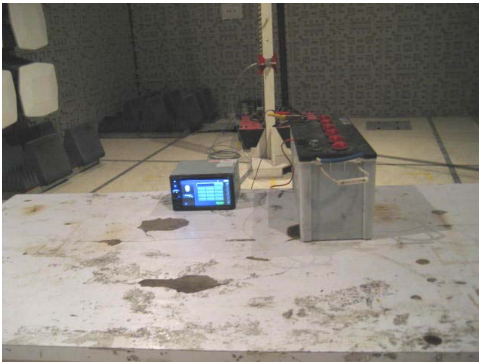
TEST SETUP OF RADIATED EMISSION (above 1GHz)
