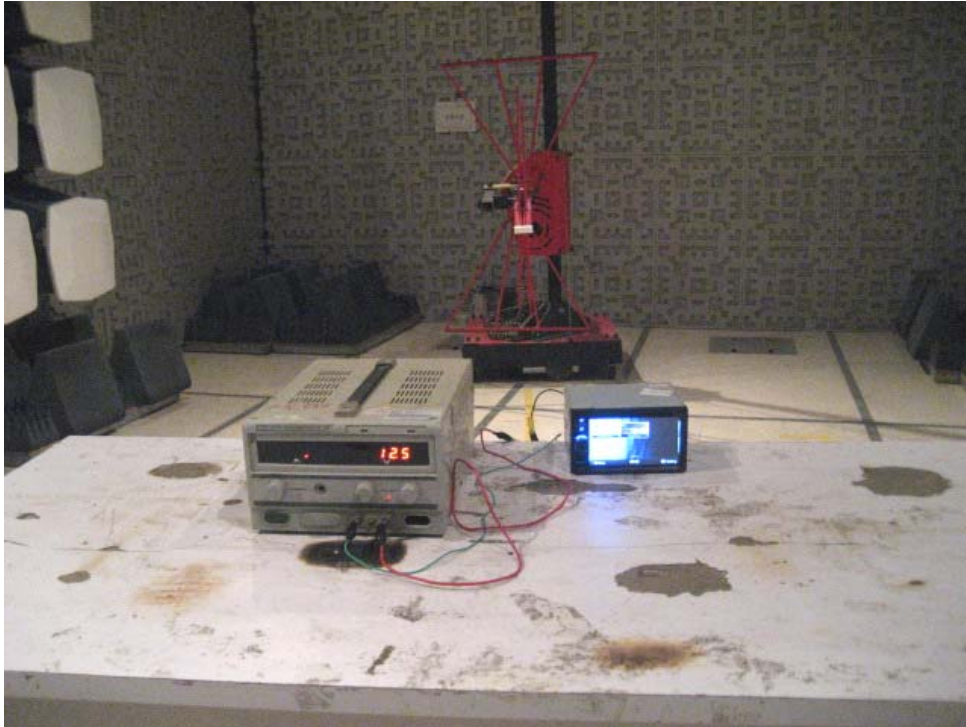
TEST SETUP OF RADIATED EMISSION (30MHz-1GHz)
