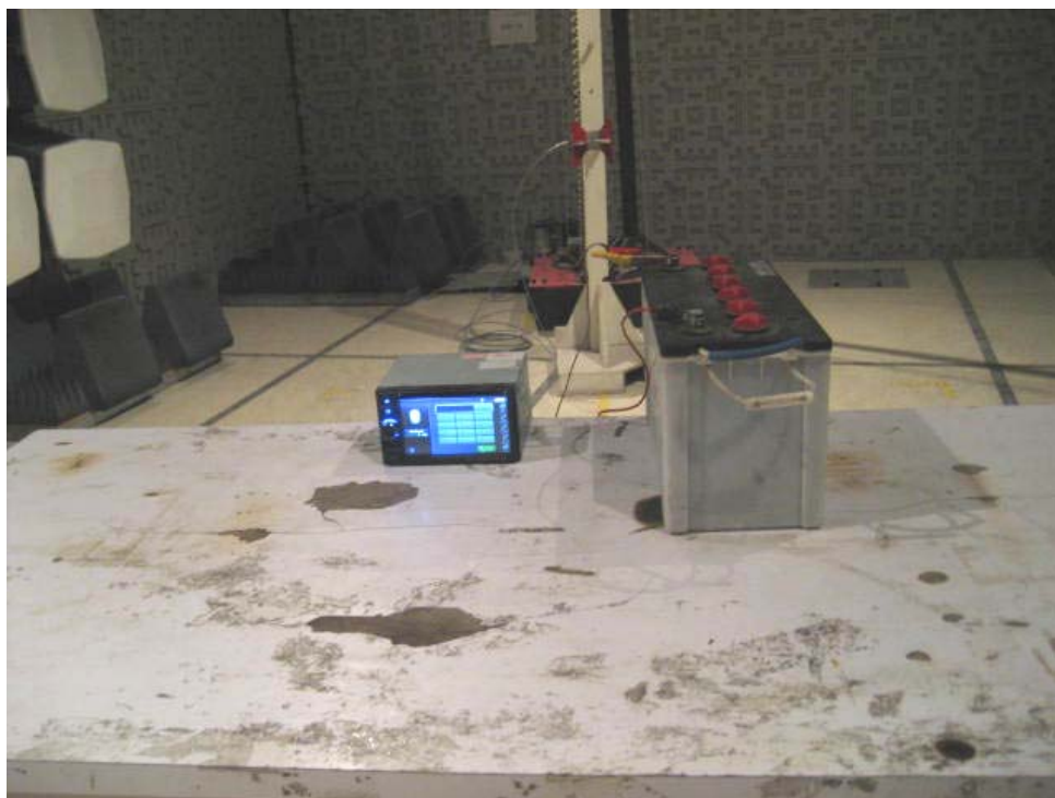
TEST SETUP OF RADIATED EMISSION (above 1GHz)
