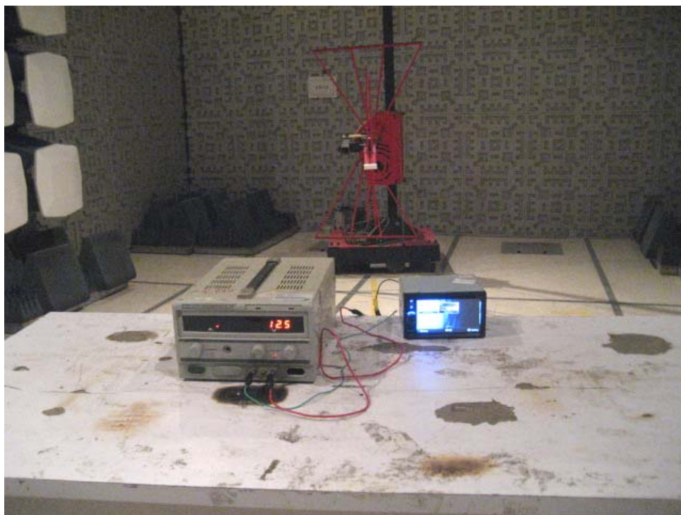
TEST SETUP OF RADIATED EMISSION (30MHz-1GHz)
