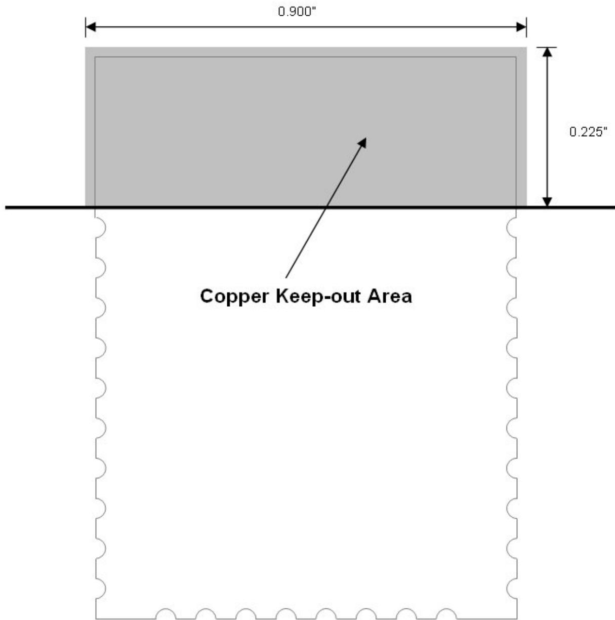
For maximum antenna performance hang the antenna keep-out area over the edge of the base board. Placing a ground plane on the layer directly beneath the WAT Module will allow you to run traces under this area. The WAT board can be placed on a base board without antenna overhang as long as all copper is kept away from the antenna keep-out area.
