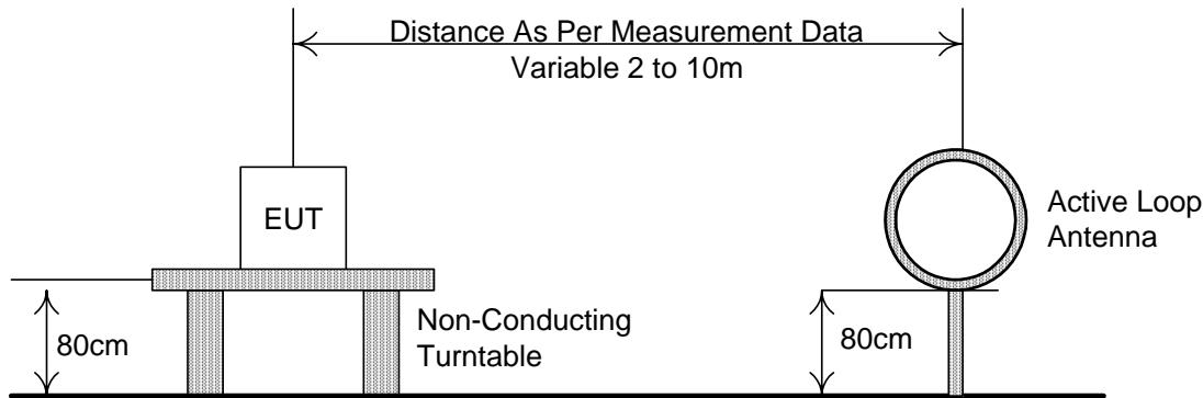
**Test Site For Radiated Emissions Above 30MHz**
