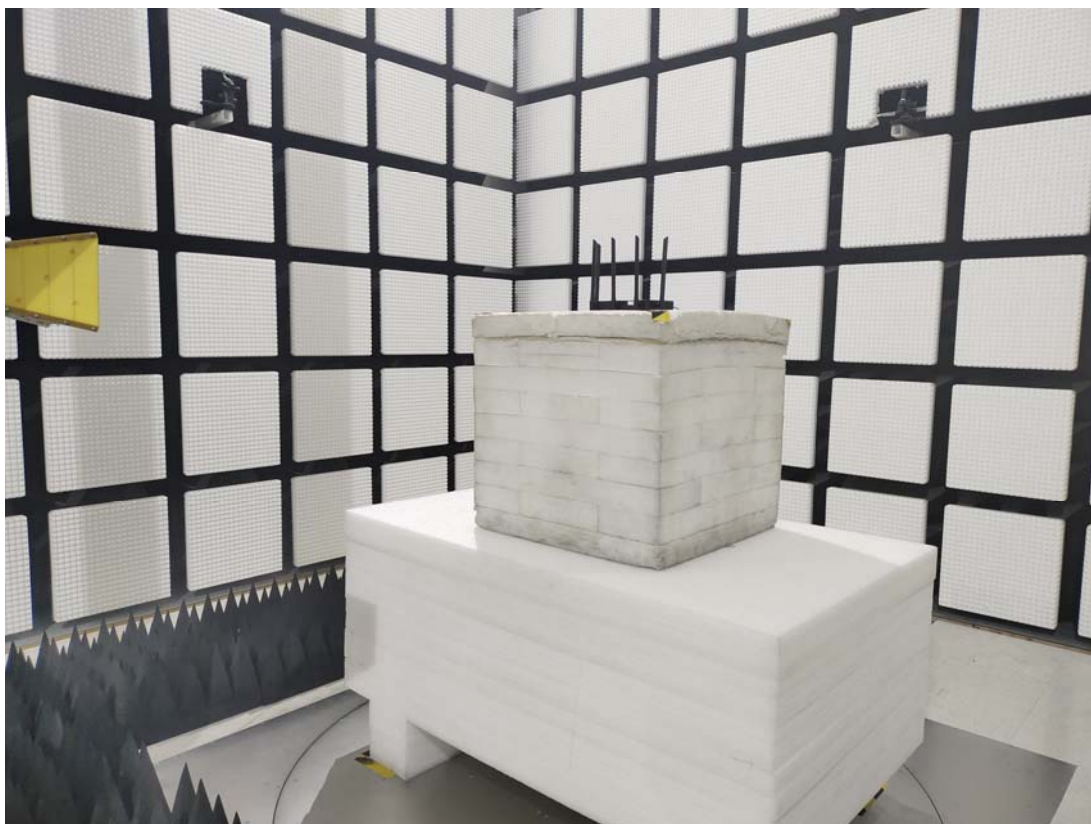
Radiated Emission Above 1GHz View
