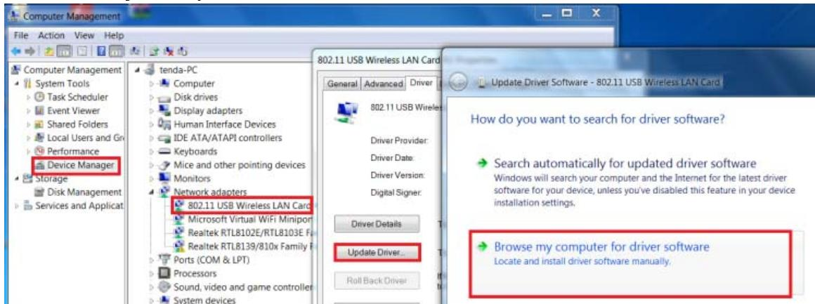
If you are using the Win7 OS that does not come with internal wireless adapter driver, do as follows:
