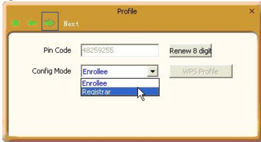
Select "Registrar" as the config mode and enter the router's PIN code, such as 35475088 that displays on the router's WPS screen in section 2.1, in the PIN code field here.
