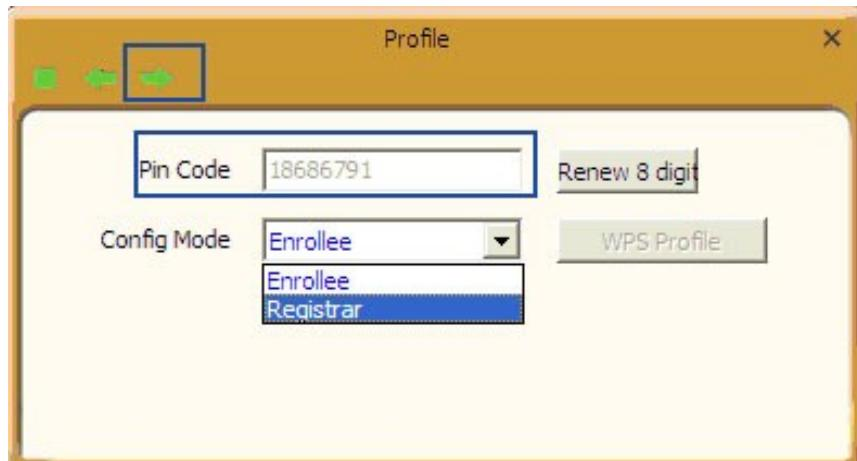
Here we take Tenda W311R as an example. First enter its WPS configuration screen, enable WPS settings and select PIN for WPS mode and then input 18686791 in the PIN code field, and then click the "Save" button. When the WPS indicator of the Router starts flashing, it indicates that WPS feature is enabled.
