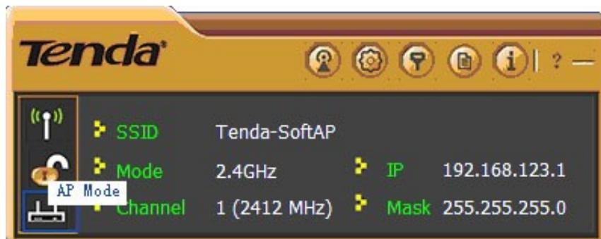
When it is switched to AP mode, the wireless adapter will automatically set its IP address as 192.168.123.1, and other clients that connected to this AP will automatically obtain the IP addresses of: 192.168.123.X(X is any integer from 2 to 254). The function buttons on the top (From L to R) are respectively Config AP, Advanced, Access Control List, Associate List, About, Help, and MiniSize, while the left
