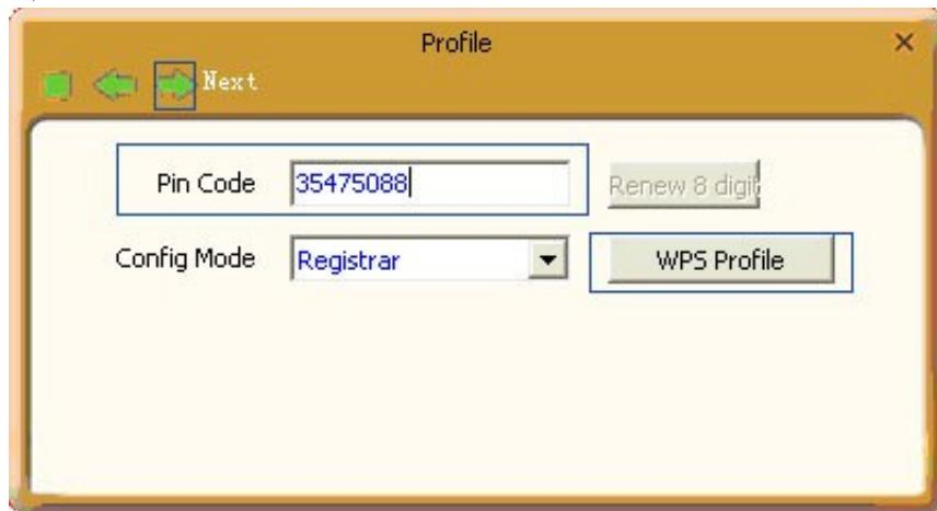
Now you can view the SSID, authentication type, and encryption type that need to be negotiated by the WPS in registrar mode. These values can be modified but we recommend using the default. Here we use the default setting and then click the next button.
