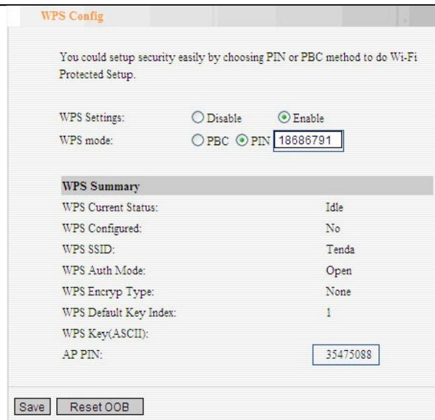
Click the next button on the Profile List screen and click “Start PIN” to start the PIN code negotiation.
