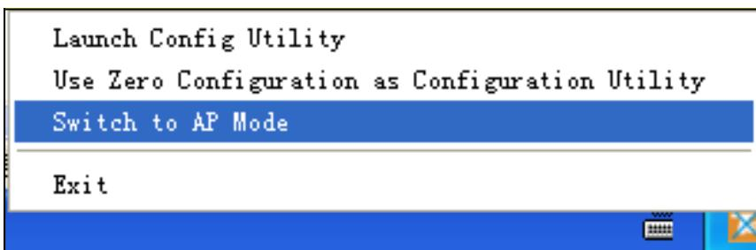
In this mode, the wireless adapter acts as an AP to transmit wireless signal and create a wireless network, while allowing other wireless clients to access this network.
