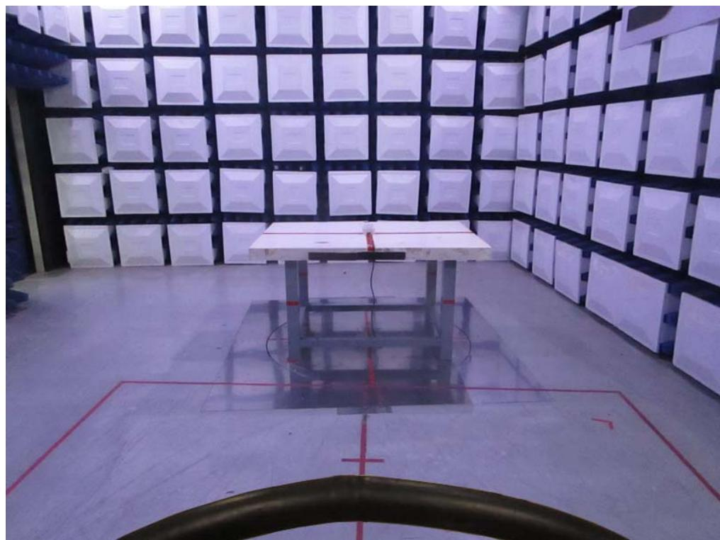
**Radiated Emissions Test Photos****30 MHz to 1 GHz**
