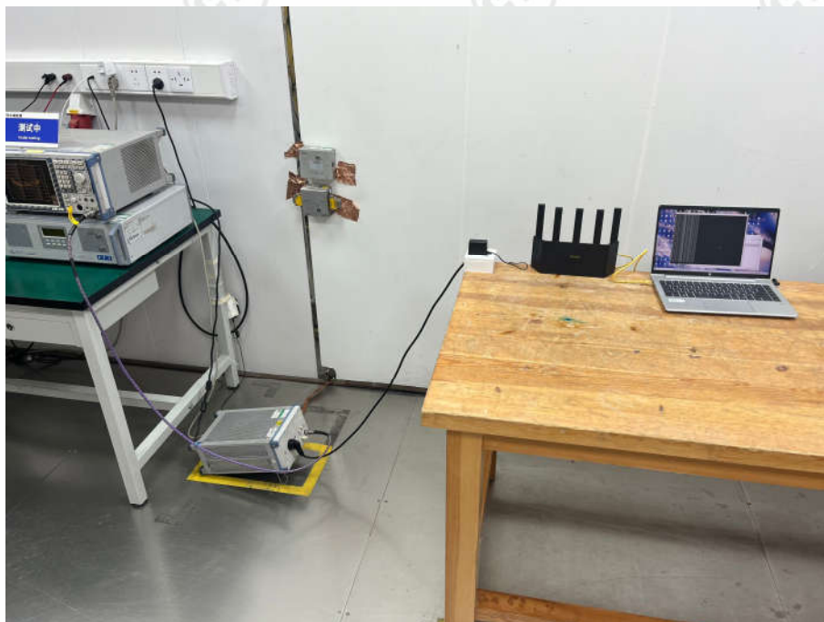
Conducted Emissions Test Setup
