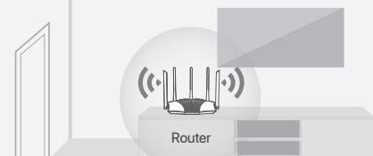
Recommended Installation: Place the extender midway between the router and the Wi-Fi dead zone.
